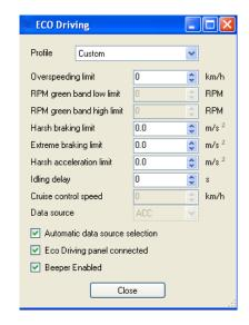
In **ECO Driving options** pop up you can select predefined **profile** for vehicle – *Truck* or *Light vehicle*. At bottom of pop up is eco driving *data source*. If you select **ACC**, unavailable parameters will grey out (e.g. RPM green band limit). Upon selection of **CAN** all parameters will be available.
